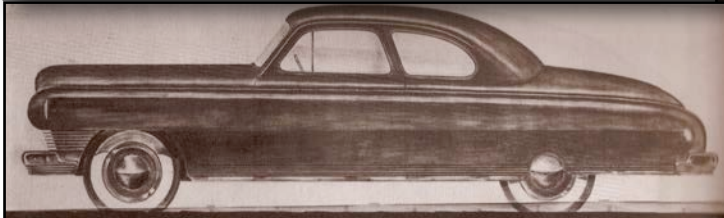
Figure 17-20. After Edsel and Gregorie settled on a design direction for an entire new line of automobiles in 1941, Gregorie began some design proposals for consideration. Well along by April 1942, this is an early fastback/boat-tail design for the "big Ford." (Photo from the Collections of Henry Ford Museum & Greenfield Village)
